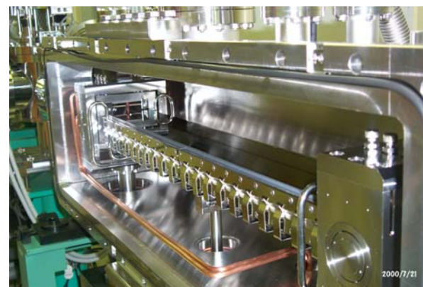
For 1-m-long mirror, vertical deflection, w/ bender, Indirect water-cooling
