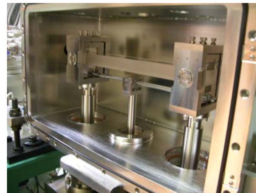
For 400-mm-long mirror, Vertical deflection, w/ bender
