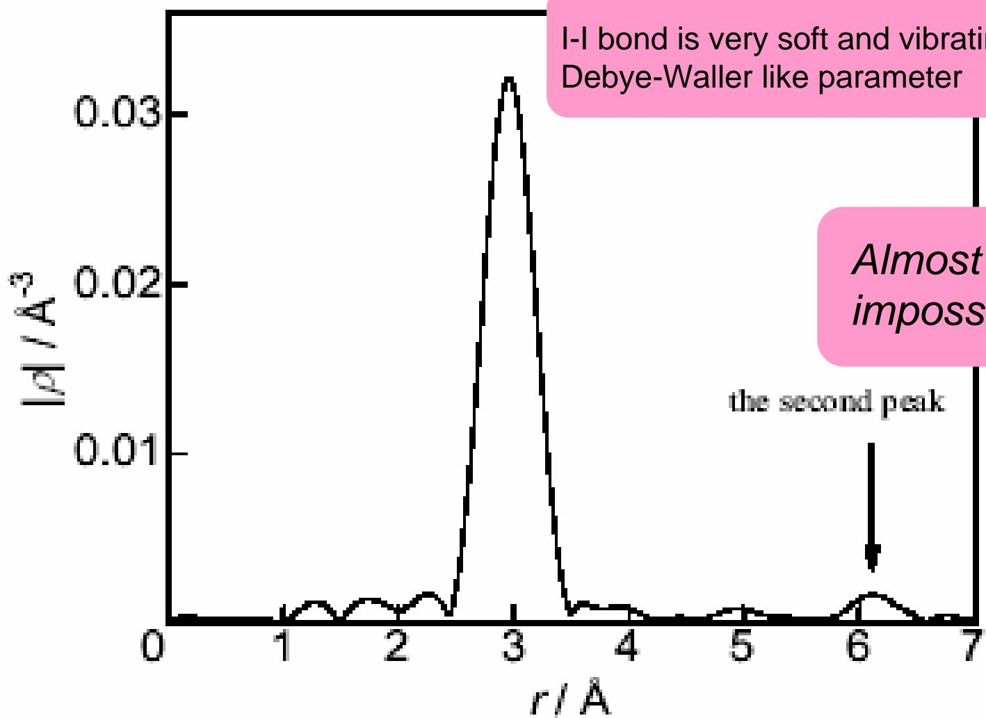
Iodine K-edge EXAFS Fourier transform for the compound spectrum made up from 12 independent spectra for organic solvent solutions.
