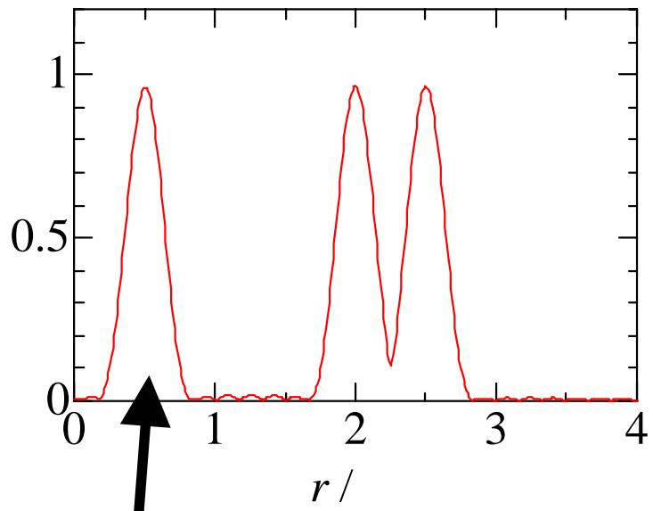
This must be a **BACKGROUND** structure, not corresponding to a real atom-atom distance.
