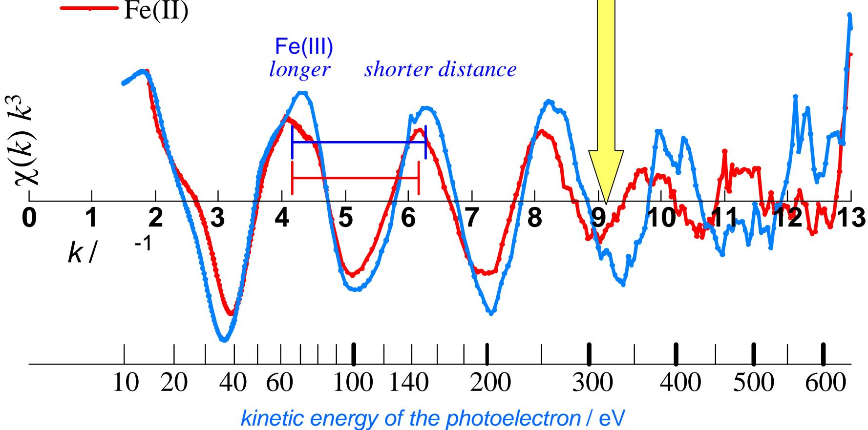
*The simplest way of knowing the wave number (corresponding to the distance) is Fourier Transformation of wave on  $k$*
