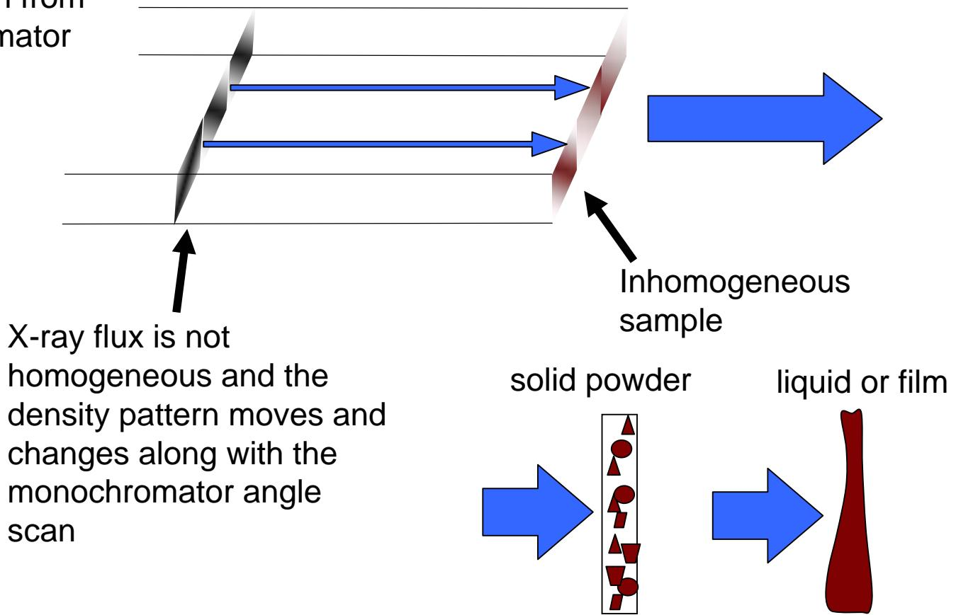
*Leads to weaker EXAFS oscillation amplitude and noisy spectrum*
