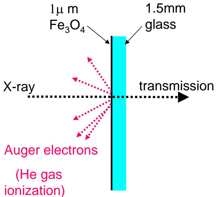
This method can be applied to thick samples owing to the short escape depth of Auger electron.
