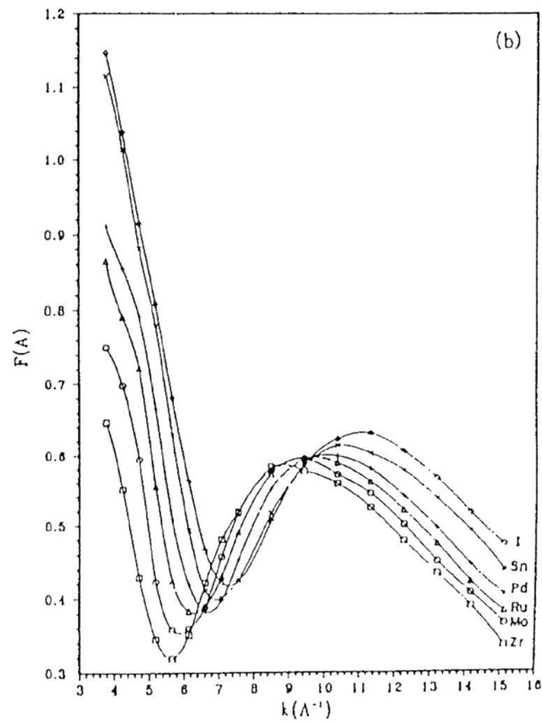
Total phase shift experienced by the photoelectron is given by  $\delta_{ij}(k) = 2 \delta_i^c(k) + \theta_j(k)$
