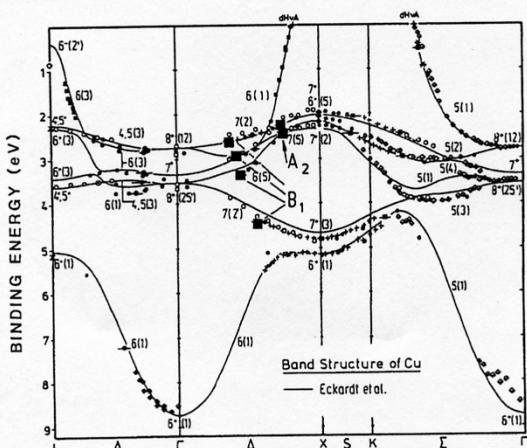
Fig.7.17. Occupied part of the band structure of Cu[7.39] with data points from various sources and a theoretical result [7.53]. Also shown (squares) are the two \$A\_2\$ points and the four \$B\_1\$ points from Fig.7.16
