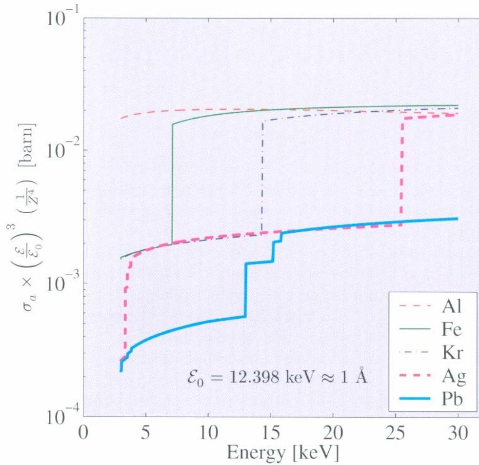
The scaled absorption cross-section as a function of photon energy for a selection of elements. The absorption cross-section per atom,  $\sigma_a$ , has been scaled by dividing it by the atomic number  $Z$  to the fourth power, and multiplying it by the photon energy  $\varepsilon$  to the third power.
