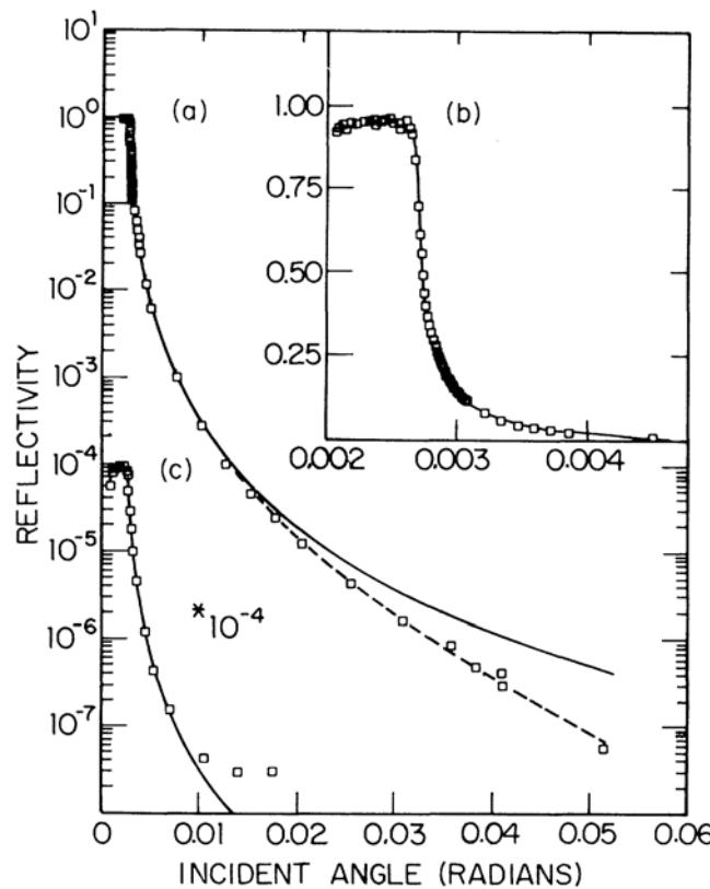
FIG. 3. (a) The measured x-ray reflectivity of water (squares) vs  $\theta$ . The solid line is the convoluted Fresnel form as described in the text. The dashed line includes  $|\Phi(Q)|^2$ . Part (b), expanded version on a linear scale for small  $\theta$ ; part (c), water reflectivity measured with use of a rotating-anode x-ray source. For  $\theta \geq 0.01$  the signal is dominated by dark counts.
