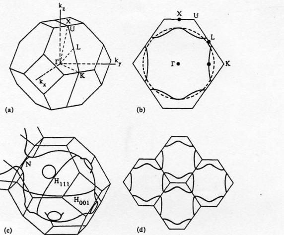
Fig. 10-15 Various aspects of the Fermi surface of Cu. (a) The Brillouin zone of an fcc lattice with some special points labeled. (b) A (110) section of the Brillouin zone. See the text for the meaning of the internal curves. (c) The proposed Fermi surface of Cu. (d) The extended zone picture of a (110) section of the Fermi surface showing the dog bone orbits.
