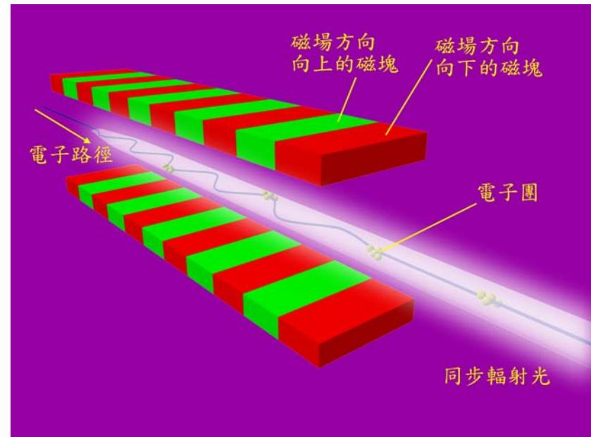
Wiggler: radiation adds incoherently ( $I \sim 2N$ , N: number of magnet periods)
