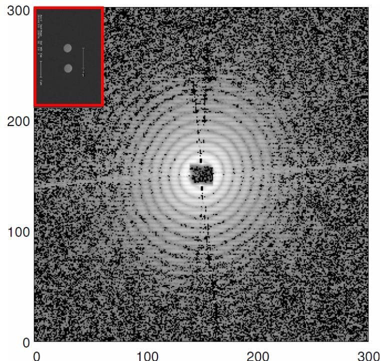
Diffraction Pattern of ~2.5 um spacing Au dots
