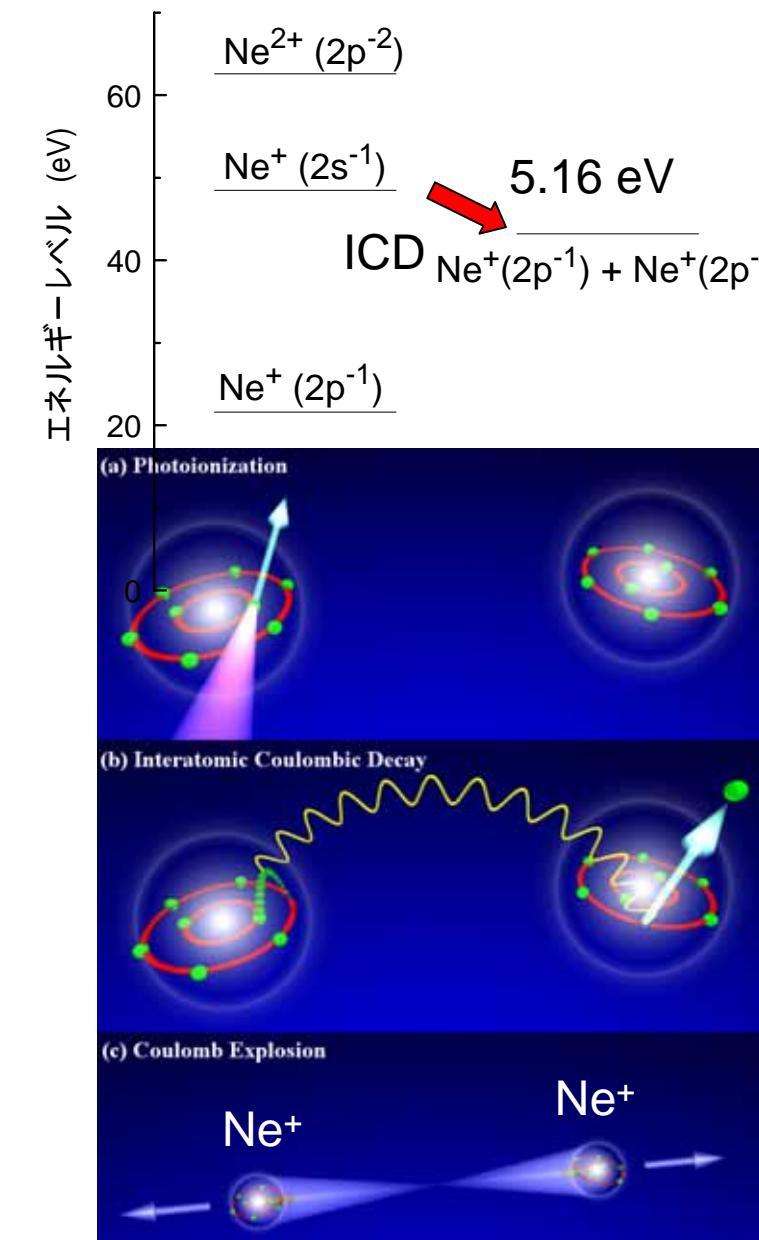
Electron-ion-ion coincidence momentum imaging
