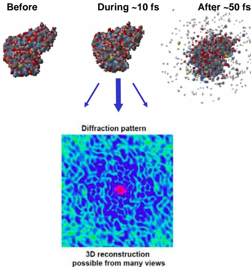
Should record the X-ray diffraction pattern before Coulomb explosion....
