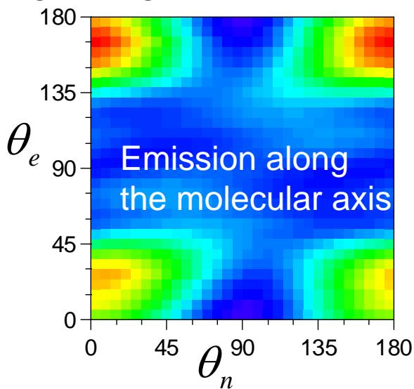
In both cases, the intensity drop at  $\theta_n=90^\circ$  i.e.  $\Sigma-\Sigma$  parallel transition.
