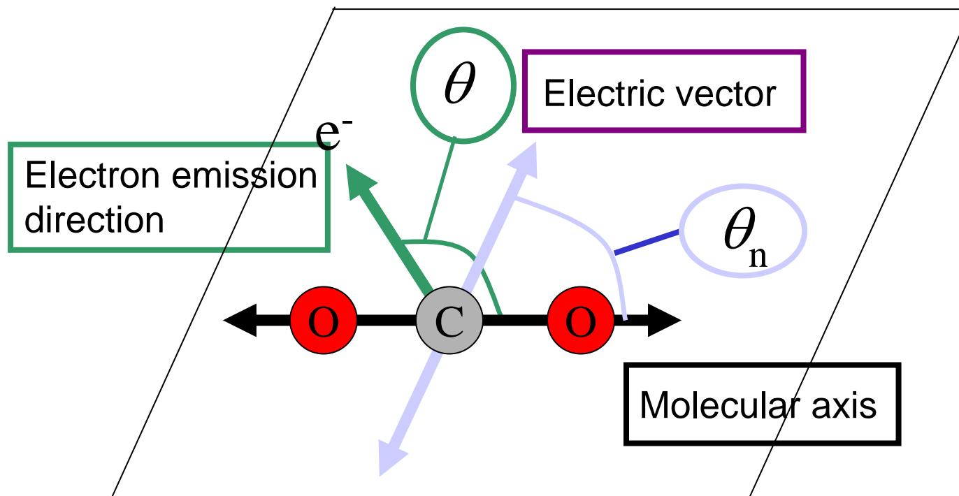
*We focus on the electron emission within this reaction plane*
