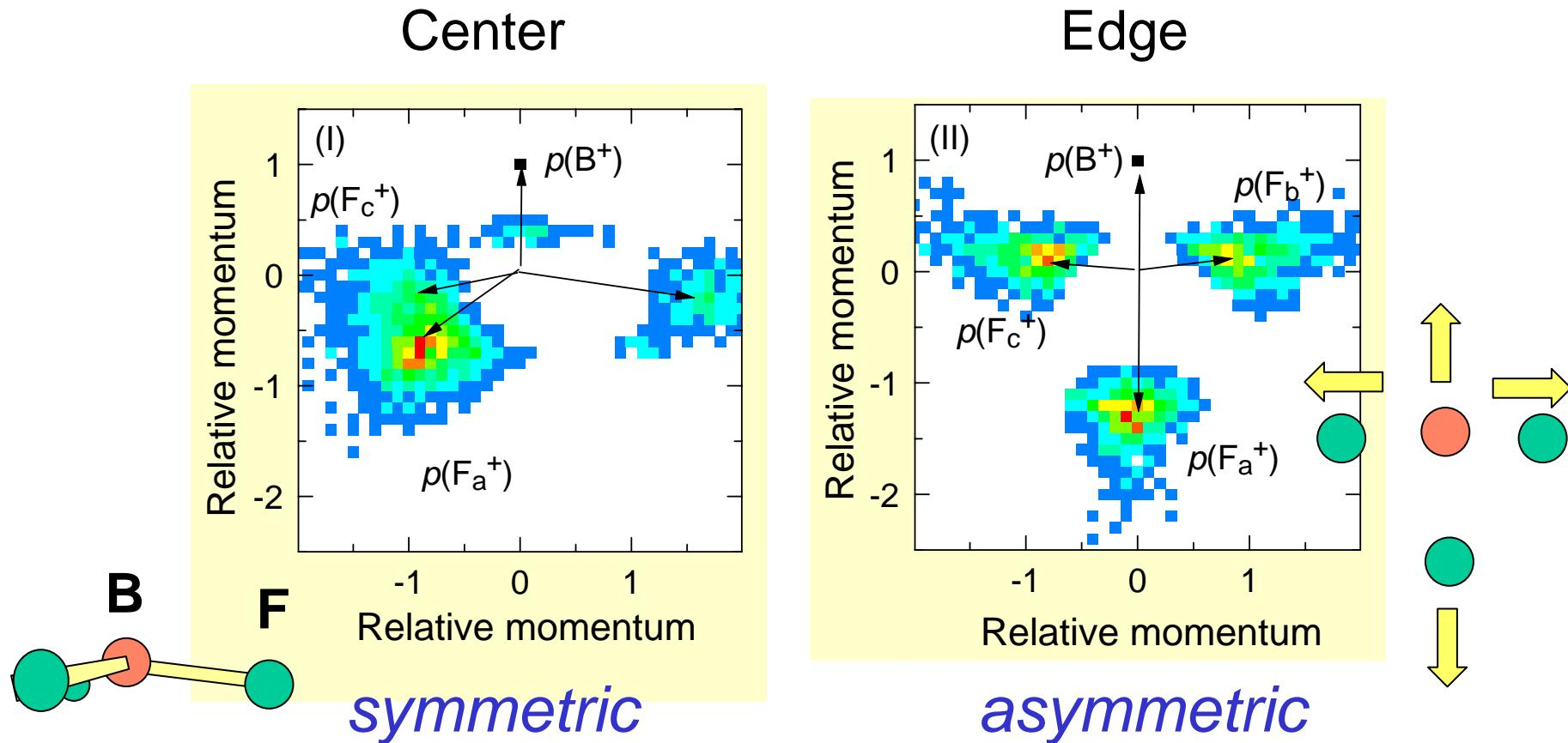
Asymmetric nuclear motion as result of symmetry breaking by F 1s ionization can be detected only via *quadruple ion momentum imaging*.
